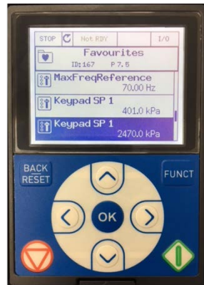
Press down arrow button to highlight Keypad SP 1 relating to condensing pressure
