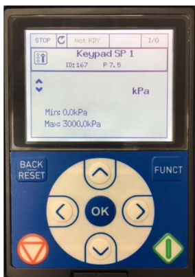
Press arrow buttons to set target pressure and OK button to confirm selection
