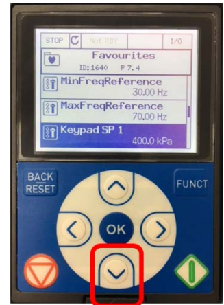
Press down button multiple times to get to Keypad SP 1 parameter relating to suction pressure and press OK
