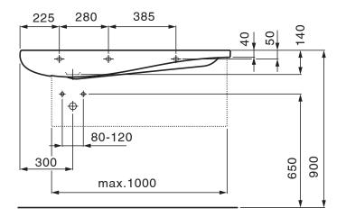
Dimensions are nominal measurements only. Dimensions shown in millimetres.
