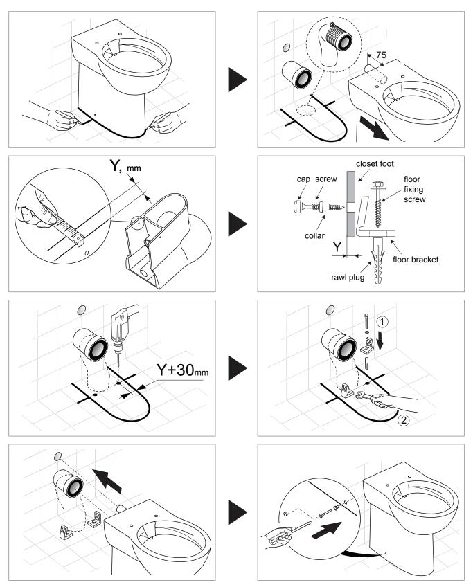
The installation of the toilet suite shall be in accordance with the normal minimum drainline grade requirements in AS/NZS 3500.2
