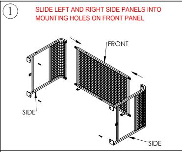
[2]USING SCREWS PROVIDED, SCREW SIDES AND FRONT TOGETHER. DO NOT FULLY TIGHTEN AT
