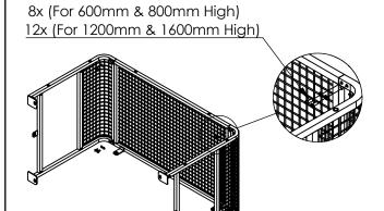
(3)JOIN TOP AND BASE PANEL TO SIDES AND FRONT. TIGHTEN ALL SCREWS ON TOP AND ON SIDES AND FRONT.
