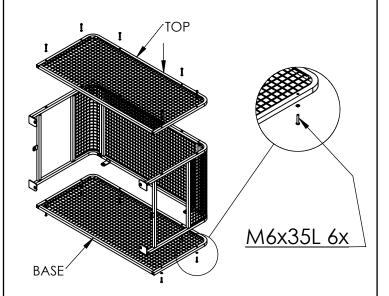
4 DOOR MAY BE PADLOCKED THROUGH EYELETS PROVIDED OR SCREWED SHUT WITH METAL DRILLING SCREWS (Metal drilling screws not provided)
