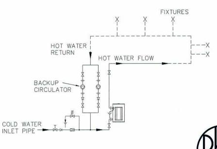
RHEEM WATER HEATERS HEAVY DUTY ELECTRIC 1 x 613050
