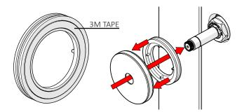
Remove the Dress Plate from the wall ensuring the Retainer is secured to the wall.
