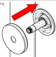
Push Handle onto Cartridge. Ensure it is level in the off position. Fasten with Grub Screw and instrall Handle Cap.
