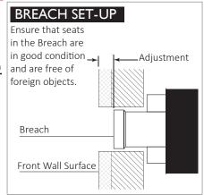
Screw Cartridge Body into recess until Catridge Seat meets a physical the Spindle and then firmly stop.
