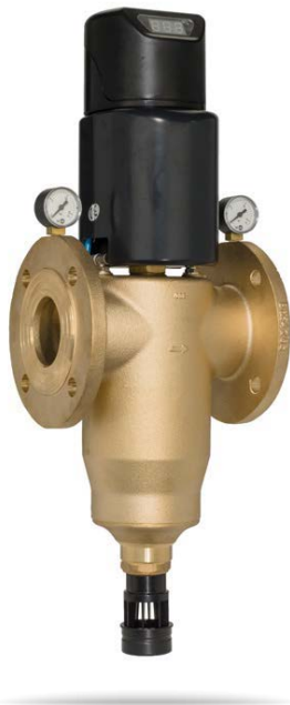
BWT Multipur AP fully automatic operation, time and/or differential pressure-controlled backwash process with drain connection for commercial applications.
