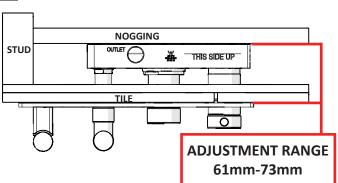
Screw the Mixer Breach onto Nogging to dimensions shown in adjustment range.
