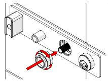
Apply Teflon tape. Tighten Hand Shower Adaptor to G1/2" thread.
