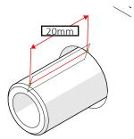
Ensure between 18mm-21mm of the Diverter spindle is protruding from the tile face. If greater trim to size using hack saw.
