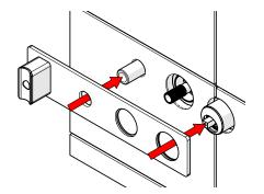
Tighten Diverter Locknut securing the dress plate.
