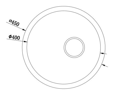
Please note that cutout template is provided as a guide only. This cutout template should be checked against actual sink unit to determine correct fit.
