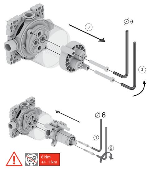
Tighten the 2 screws parallel (1 turn each side) Check before installation that all seals are available and at the right place
