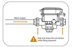
**Note:** Brace this fitting to prevent movement while connecting to the mains supply.
