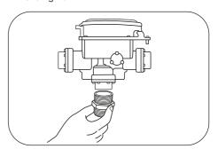
**Note:** If you cannot screw the switching unit on top of the barrel union due to space limitations, you can unscrew the barrel union nut and release the nipple from the union. Rethread the nipple into the switching unit making sure the union nut remains on the nipple. Re-join the union to complete connection.
