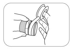
Thread the nipple into the base of the switching unit until it is watertight. Do not overtighten.
