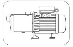
**Note:** It is recommended the pump should be no further than 3 metres from the tank.
