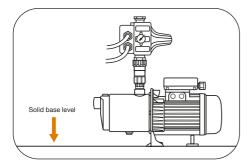
**Note:** If you are installing the VFB-APC directly onto the Horizontal Multistage Pump, use a 25mm barrel union. If you are installing the VFB-APC between the pump and first outlet, use pipework with a minimum internal diameter of 25mm.
