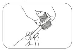
Thread the nipple into the female socket of the pump discharge until it is watertight. Do not overtighten.
