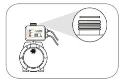
Hold the Mechanical Switching Unit (VFB-MSU25) over the outlet and connect the loose nut. Do not overtighten. The rubber washer will lock this in place.
