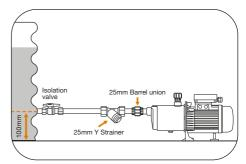
**Note:** The length of the suction pipe should only run between 1–2 metres.
