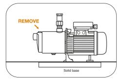
Slowly open the tank isolation valve allowing water to fill the suction line and pump casing. This will expel the air as the water fills the suction line and pump casing.
