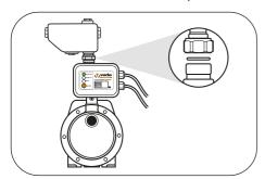
3. Connect the mains water pipe to the VFB-MSU25 outlet labelled "mains in".
