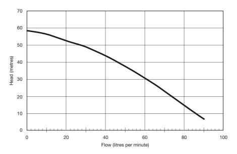
**Note:** The curve above represents the pump with the VFB-APC.
