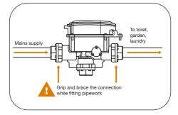
9. For easy maintenance install an isolation valve on either side of the VFB-DSU.
