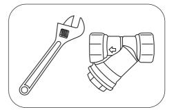
2. Use a steel brush to clean the dirt from the filter.
