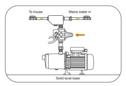
3. Using a flat head screwdriver, turn the adjustment screw clockwise until you reach the correct pressure (roughly, this will be 3.5 full 360° turns).
