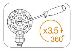
Confirm the pressure has been correctly adjusted by slowly opening an outlet and checking the gauge on the side of the VFB-APC. If the pump starts when the gauge drops to 2.2 bar the cut in pressure has been successfully adjusted.
