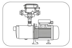
Connect the 25mm female end of the switching unit to the incoming mains water supply. This is marked 'MAINS' with an arrow pointing out of the VFB-DSU (indicating water flow direction).
