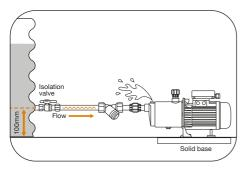
Close the isolation valve and replace the priming port plug. The isolation valve must be re-opened prior to operation. Your pump is now primed. Before pump operation ensure there is sufficient water inside the tank.
