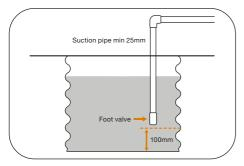
Connect the suction pipe to your Horizontal Multistage Pump. Ensuring both an inline filter and barrel union have been installed in the suction line. The inline filter prevents dirt and debris entering the pump and will prolong product lifespan.
