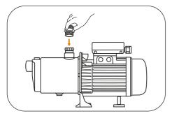
Connect the 25mm female end of the barrel union to the nipple until it is watertight. Do not overtighten.
