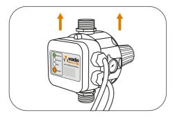
Check the set up so far. Ensure that the VFB-APC is braced or fixed so minimal movement occurs once in operation. If the distance between the pump and highest outlet exceeds 15m, adjust the cut-in pressure on the VFB-APC.
