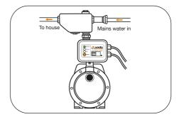
For easy maintenance down the track, install an isolation valve into both the mains and house water line.
