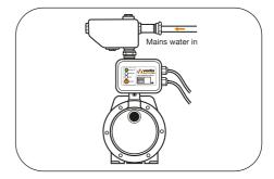
4. Connect the house water pipe to the VFB-MSU25 outlet labelled "to house".
