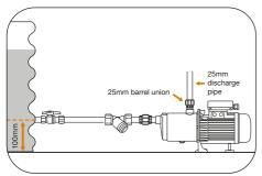
**Note:** It is crucial that you use the recommended pipe size until at least the first pipe branch (T piece) is reached.
