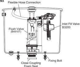
Note: Stop Valve and Flexible Hose with Elbow supplied with Back Inlet variant.
