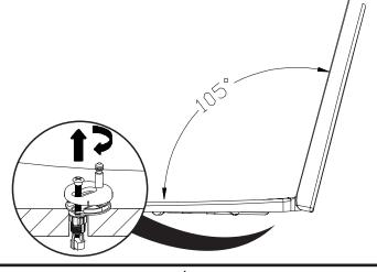
**3.** Fix toilet seat, align onto hinge pins.
