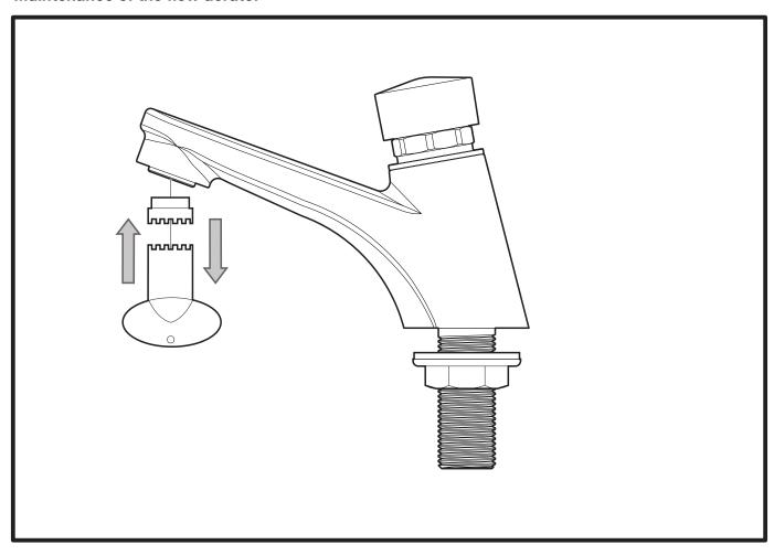
Note: For cleaning and maintenance of aerator, use key provided to remove and replace. Cleaning may be required if there is a noticeable reduction in flow.
