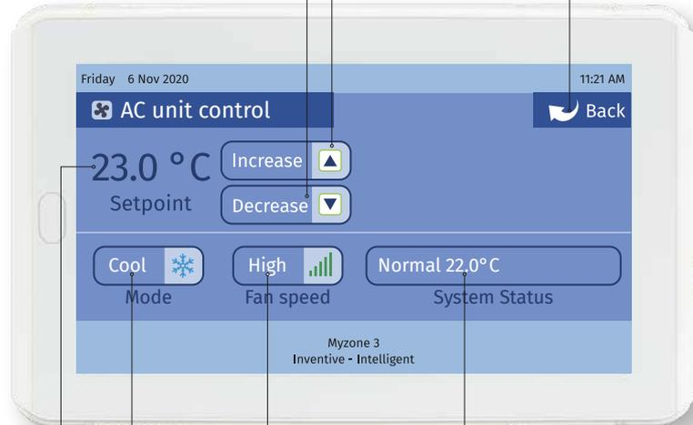
Current A/C unit set point (If unit is set to control from the Return Air). If unit is set to control from zones this will show the current zone controlling the outdoor unit. \*Check with your installer to determine if unit is controlling from Return Air or Zones.
