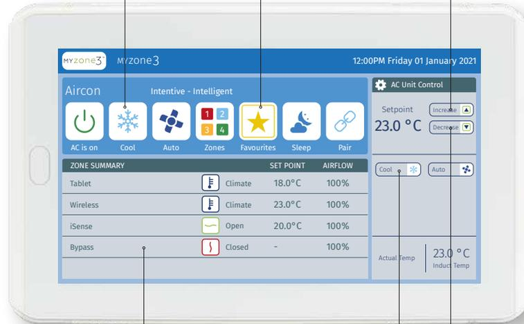
The zone summary provides an overview of the zone names, current setting for the zone and airflow for the zone
