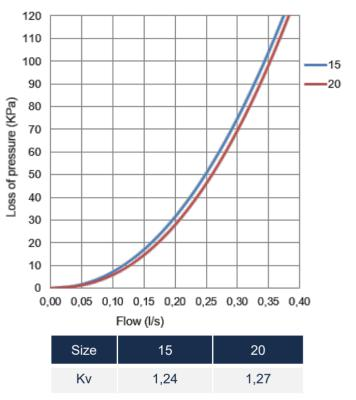
Kv (m3/h), cubic meters per hour that flow through the valve generating a loss of pressure of 1 bar.
