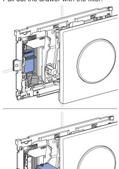
Dispose of the drawer with the filter and have a new drawer ready.
