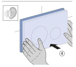
✓ The LED behind the actuator plate goes out.
