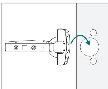
With top cover plate lifted, place hinge into position on door and insert into holes until flush.
