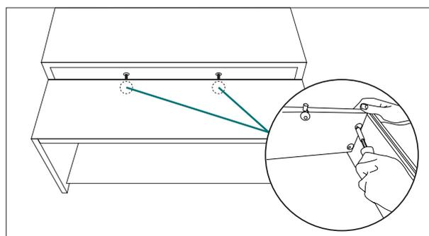
Carefully lay vanity unit on its back on a flat surface. Using the pre-drilled holes at the base of the unit as a guide, insert the cam-locks at the top of the kickboard and fasten to vanity unit.
