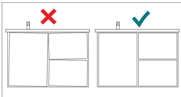
Install drawers and doors back onto cabinet and make adjustments to align the doors and drawers correctly.
