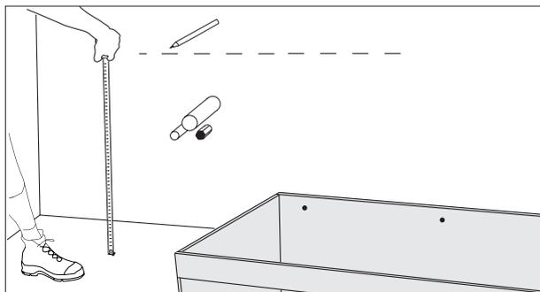
After completing the Prior to Installation Checklist, mark the position of the top of the vanity. Don't forget to factor in the top/basin thickness to get the correct height.
