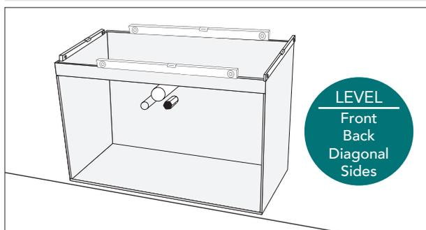
Position the vanity over the pipes in the correct position and fix with a single screw in centre of vanity to hold in place.
