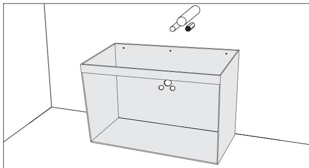
Remove doors and drawers. Measure correct plumbing locations and drill holes for plumbing in the back panel and/or base of the cabinet with an appropriate sized hole saw. Pre-drill screw locations for fastening to wall.
