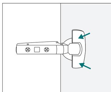
Once secured in position, click cover plate down to lock into place.
