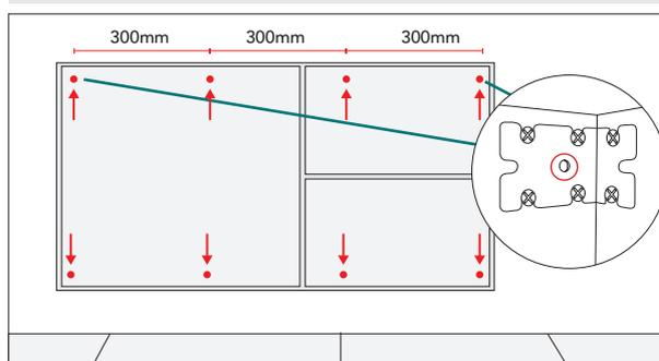
Securely fasten the vanity to the wall through back of vanity with appropriate screws/bolts at TOP and BOTTOM of cabinet. Fix the cabinet through the top left and right hand brackets and evenly space apart the horizontal fixings at a maximum of 300mm apart. For the bottom start the fixing points no further than 100mm from each end of the cabinet and no higher than 50mm from the base panel.
