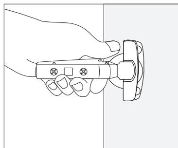
Pull hinge up and out from door. You may need to wiggle the hinge to loosen and use a little force.
