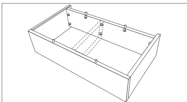
For larger units (1200mm and bigger), insert the centre support panel supplied and secure all cams.
