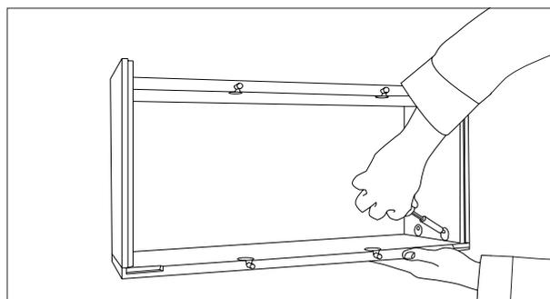
Attach and fasten the front panel to each side panel. Ensure all cam-locks are fastened.
