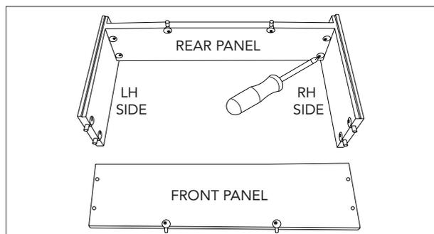
Join each side panel with rear panel. Use a phillips head screw driver to fasten the cam-locks clockwise into the pre-drilled holes.
