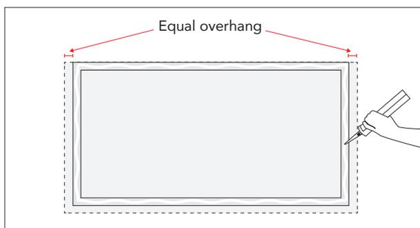
Using a non-acidic silicone, apply a continuous bead of silicone to the top four edges of the vanity and at the back where the top meets the wall. Position the top so it has equal overhang on each side, ensuring the top surface is level.
