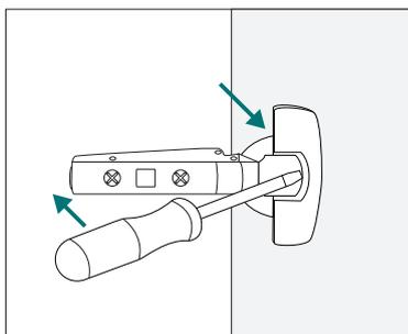
Once you have removed door from the cabinet, using a flat head screw driver, lift and release the top cover plate.
