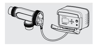
Plug the Henden Compact Salt & Mineral Chlorinator 3-pin plug into a suitable weatherproof RCD-protected 10amp outlet.
