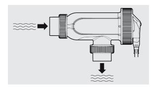
Using the reducing bushes provided, connect the Chlorinator Cell horizontally in the return line to the pool. Ensure you use high pressure cement.
