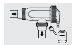
Handy tip: Check that the O-ring is clean, greased with silicone grease and securely located in the Cell Housing. Do not grease with petroleum-based jelly.
