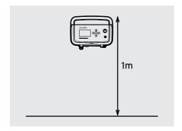
Using the mounting bracket, green plugs and screw provided, mount the Henden Compact Salt & Mineral Chlorinator onto the pool pad.
