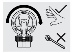
Connect the cell lead from the Henden Compact Salt & Mineral to the Cell cap. Ensure a firm fit to prevent water entry.
