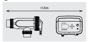
Ensure the housing is positioned in line with this illustration. This positioning will mean less water hammer on the cell plates over time and improved product lifespan.
