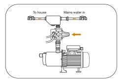
Using a flat head screwdriver, turn the adjustment screw clockwise until you reach the correct pressure (approx 3.5 full 360° turns).
