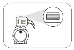
Hold the Mechanical Switching Unit (VFB-MSU20) over the outlet and connect the loose nut. Do not overtighten. The rubber washer will lock this in place.
