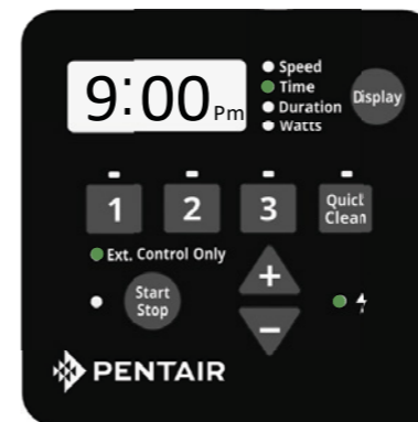
Figure 12: Activating External Control Only
