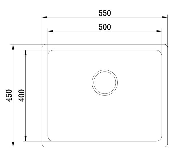
Please note that cutout template is provided as a guide only. This cutout template should be checked against actual sink unit to determine correct fit. 430mm
