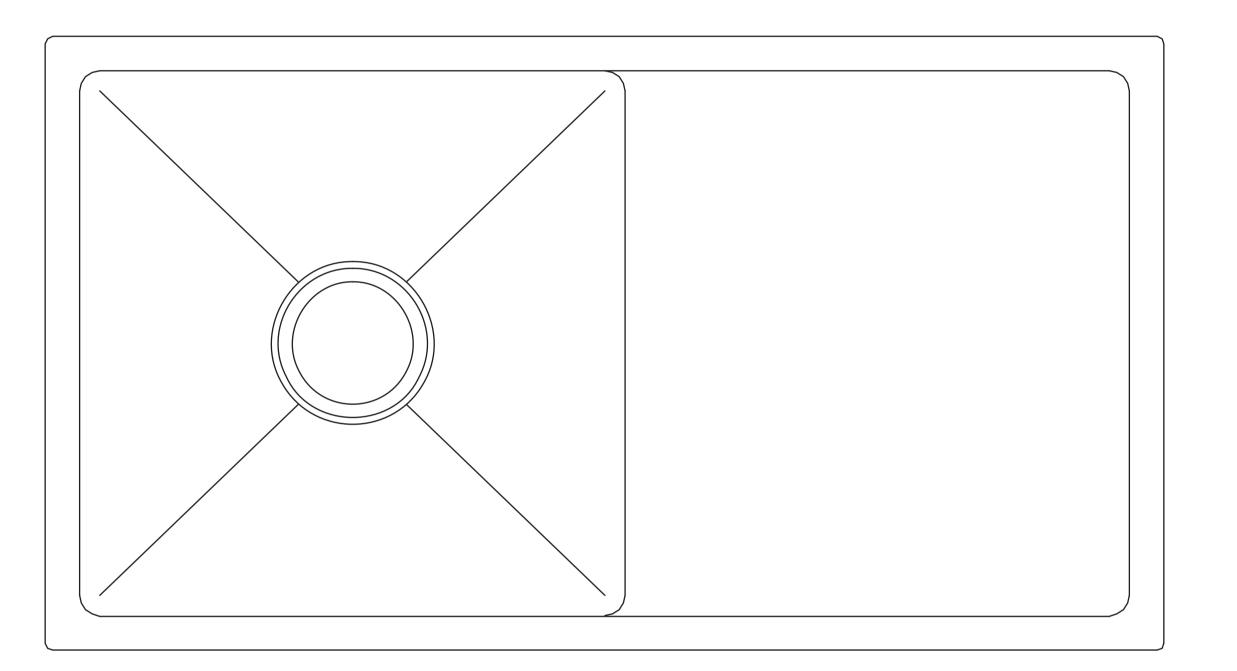
Use inner line for undermount installation Use outer line for inset installation
