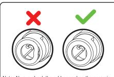
Note: Always check the rubber seal on the ceramic Cartridge is a round uniform shape. If distorted push back into place or the cartridge will leak when water is introduced.
