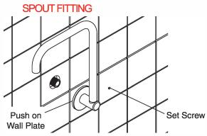
Remove the set screw from the rear of spout assembly and place somewhere safe. Carefully place the push on wall plate onto the assembly if not already done so.
