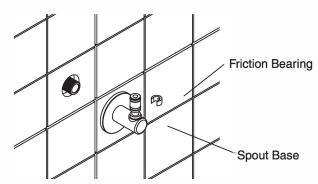
Remove the friction bearing to avoid any risk of loss or damage while fixing and tightening the spout base.
