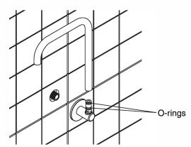
Remove the spout being careful not to damage it or the o-rings.
