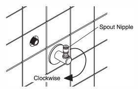
Apply a sufficient amount of a good quality thread sealant and in a clockwise direction screw the spout base onto the outlet until base is flush with the wall and the spout nipple in a verticle position. Ensure seal is achieved then push the push on wall plate gently against the finished wall. Re-assemble the spout assembly to complete the installation.
