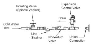
Note: a combined isolating valve/non-return valve/line strainer may be used.
