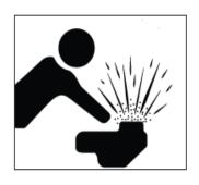
WARNING – Hazardous Pressure. Pool and spa water circulation systems operate under hazardous pressure during start-up, normal operation, and after pump shut-off. Stand clear of circulation system equipment during pump start-up. Failure to follow safety and operation instructions could result in violent separation of the pump housing and cover due
