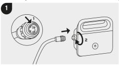
Attach the floating cable to the power supply.
