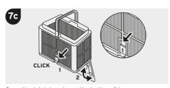
Open the latch to release the bottom lid.
