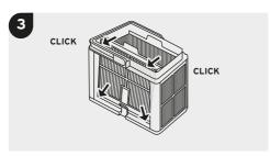
Reassemble the filter panels.
