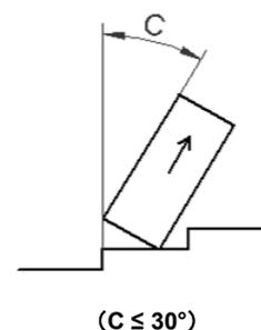
In addition, tilting the water heater more than 30° from the vertical during handling will unsettle the refrigerant gas and compressor lubricating oil. If the water heater has been tilted, it will need one hour to settle before the power to the water heater can be switched on, otherwise damage to the compressor may result.
