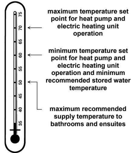
We recommend and it may also be required by regulations that an approved temperature limiting device be fitted into the hot water pipe work to the bathroom and ensuite when this water heater is installed. This will keep the water temperature below 50°C at the bathroom and ensuite. The risk of scald injury will be reduced and still allow hotter water to the kitchen and laundry.
