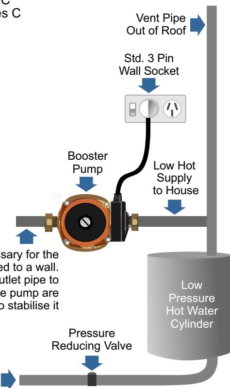
It is not necessary for the pump to be fixed to a wall. The inlet & outlet pipe to and from the pump are sufficient to stabilise it
