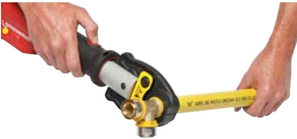
11. Press the switch mechanism until the joint is completed and the piston has retracted back into the body of the tool.
