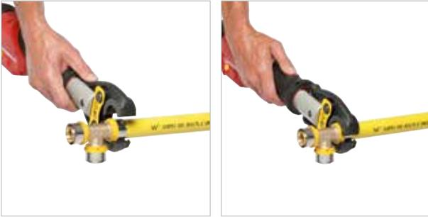
10. With the jaws open place the fitting inside the jaws so that the raised section of the plastic sight ring fits into the slot in the jaws. Release the jaws so they fit snugly over the fitting, ensuring that the raised section of the plastic sight ring is still located in the slots in the jaw.
