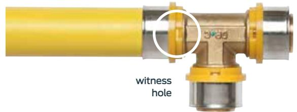
8. Insert the pipe into the fitting and under the stainless steel ring and push the pipe until it is visible in the slots of the plastic sight ring (witness hole). This ensures you have pushed the pipe home.
