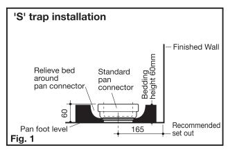
**IMPORTANT:** ALL DIMENSIONS ARE TO THE UNDERSIDE FOOT LEVEL OF THE PAN. IT IS IMPORTANT TO MAKE A HEIGHT ALLOWANCE FOR BEDDING.
