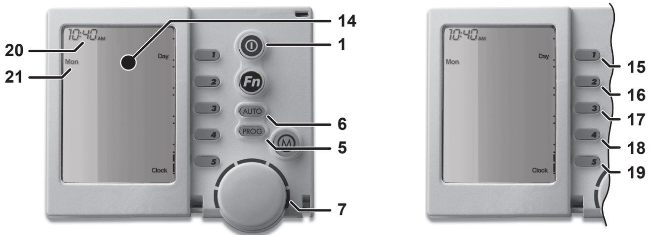
1. Ensure the Networker is turned OFF using the ON/OFF button (1).
