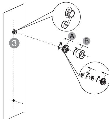
Screw inlet connector to the water supply pipe.
