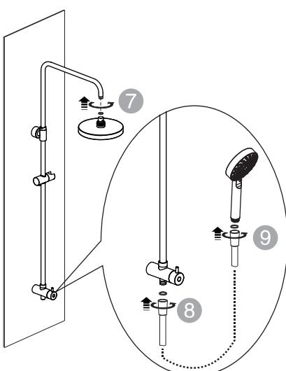
Screw shower head to bent tube, connect shower hose to hand shower and Adapter.
