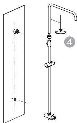
Fix the bent tube to the upper bracket as per diagram 4. To ensure upper bracket is positioned correctly the grub screw must be positioned underneath.
