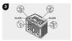
Reassemble the 4 filter panels.
