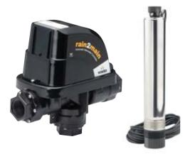
Coupled with the Vada Rain2Main, the Vada V75-S pump is the premium automatic rainwater control system. The V75-S is designed for many years of reliable service where absolute silence, high pressure and solid reliability are required. The Vada V75-S pump sits inside the tank while the Vada Rain2Main component is mounted outside the tank. If the tank is empty, the Vada Rain2Main will revert to mains supply.
