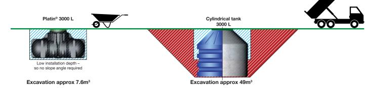
\*Based on a vertical, cylindrical tank with a useable volume of 3000 ltr, a height of 1.90m and a diameter of 2.20m. Calculation of excavation is under consideration of a ditch bottom of 10cm, a sidewise distance of 50cm and a slope with 45° gradient.
