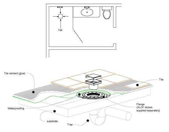
NOTE, this method requires the channel system to be above and separate from the waterproofing
