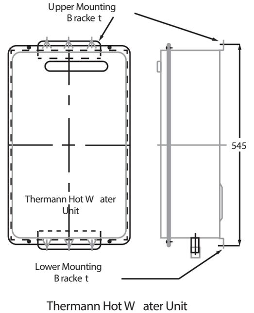
The location of the Recess Box installation must comply with AS 5601
