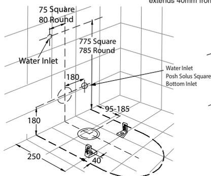
**NOTE:** Ensure back inlet connection extends 40mm from finished wall
