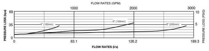
Note: The pressure losses depicted in the tables are for the device only and not the complete assembly.
