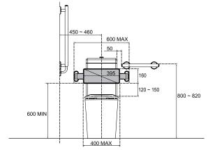
Reposition oval flange cover on mounting plate and tighten grub screw to secure Backrest.
