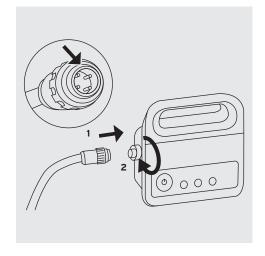
Plug the H3 power supply into the powerpoint and turn the power point on.
