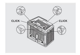
Insert the clean filter basket and close the filter cover. The filter basket handle will automatically fold down as you close the cover.
