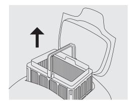
Open the latch to release the bottom lid in order to remove the debris.
