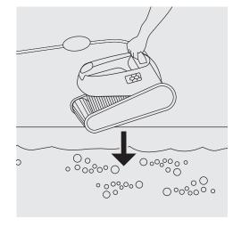
Press the ON button. The LEDs will turn on and it will start to operate. If no program is selected, it will perform a single cleaning cycle. Note: the power supply will turn off automatically after 3 hours.
