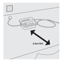
Position your H3 Robotic Pool Cleaner near your power supply unit. Unwind the cable and stretch it out completely so that it has no kinks.
