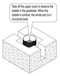
2. Cut slots according to the diagram below, note the depth includes tiles' thickness.
