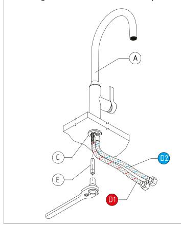
2) Fit the Hot (D1) and Cold (D2) flexible hoses under the bench and affix to Sink Mixer Assembly (A). Tighten by hand, ensure the O-rings on the flexible hoses are properly seated
