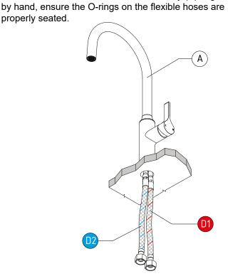
4) Connect the Hot (D1) and Cold (D2) flexible hoses to 1/2" BSP pipework and tighten firmly with a spanner. Ensure hoses do not twist or kink during tightening. Sussex recommends using Stop Cocks/Mini Stops, however, these are not supplied.
