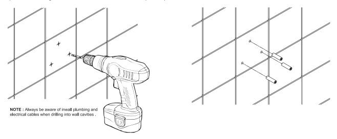
Fix the mounting brackets firmly in place using the screws supplied ensuring it is flush and firmly agains the wall.
