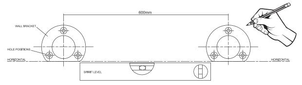
Carefully drill 7mm holes in the previously marked positions and insert the wall plugs until flush with the wall. (To ensure accuracy, we recommend to use the wall bracket as a guide and drill pilot holes using a 4mm drill bit prior to drilling the 7mm finished hole size required.)
