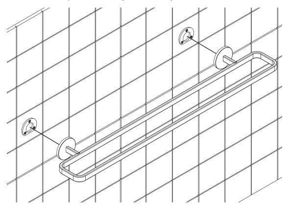
Hold the assembly in place while you **evenly** do up the two securing set screws to complete the installation.
