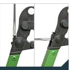
Manual tools available for copper crimp ring connections 16, 20 and 25mm. Only Auspex approved tools can be used.
