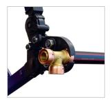
When using a battery tool, ensure the tool has fully closed and released indicating a completed joint.
