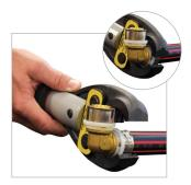
Press the switch mechanism until the joint is completed. Press the back end of the jaws and remove the completed joint.
