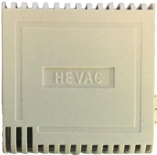
*The SRTA-DSP is an averaging type, adjustable setpoint room sensor to be used in pairs (wired in parallel). It is intended for use with Hevac brand HTC 3, 5 and Digital series controllers. The sensor has a NTC characteristic (increase in temperature = decrease in resistance) and changes approximately 160 ohms per degree. Both a concealed and exposed adjustment knob are included, allowing plus or minus 3.5°C from the HTC's main setpoint.*
