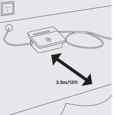
Position your H2 Robotic Pool Cleaner near your power supply unit. Unwind the cable and stretch it out completely so that it has no kinks.
