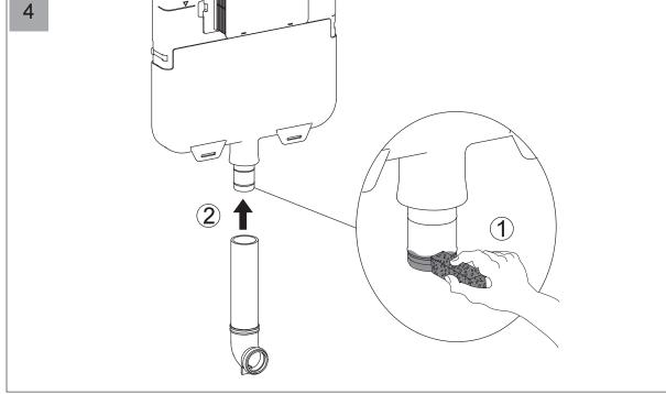
Please note: Flush pipe must be fixed securely to a cross beam inside the wall to avoid dislodging from the cistern when pan is fitted.
