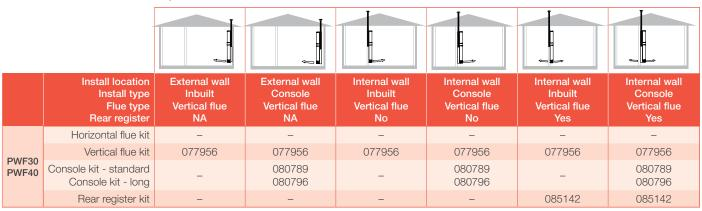
Console kit - standard: up to 3.3m ceiling height Console kit - long: up to 4.0m ceiling height
