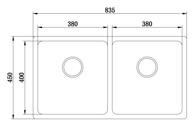
Please note that cutout template is provided as a guide only. This cutout template should be checked against actual sink unit to determine correct fit.
