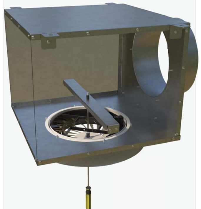
Figure 5 - Installation of a manually adjustable HSC-AD into a plenum box using a central fixing bolt with decorative cap. Suitable for sizes DN250-DN500 with manual adjustment only.
