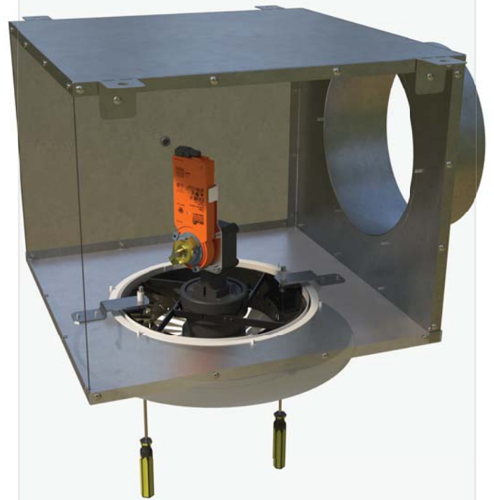
Figure 4 - Installation of an HSC-AD (shown with electric adjustment) into a plenum box using 2 bolts accessible through the diffuser face. Suitable for sizes DN250-DN500 with electric, thermal or manual adjustment.
